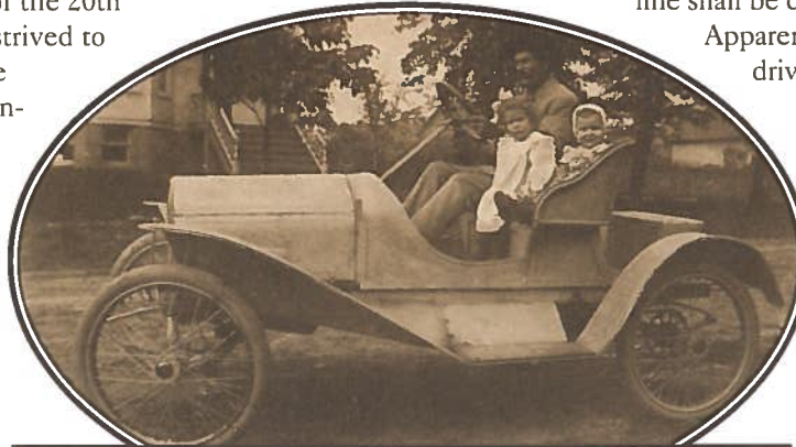
DR. MILEY AND HIS 1909 METZ RUNABOUT — Dr Miley assembled this 1909 vehicle himself. Known as the "Metz Plan", parts were shipped in 14 separate packages, each costing $25, from the factory in Waltham, Massachusetts. The owner assembled the vehicle in stages as each package arrived. The Metz Runabout had a dual chain drive.
